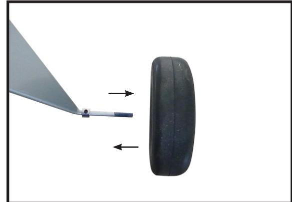
Thread a mounting screw into each of the holes to cut threads in the surrounding wood. Apply a small amount of thin CA to harden the threads made by the screws. Position the landing gear so it rakes forward. Use the screws and landing gear straps to secure the landing gear to the bottom of the fuselage.
