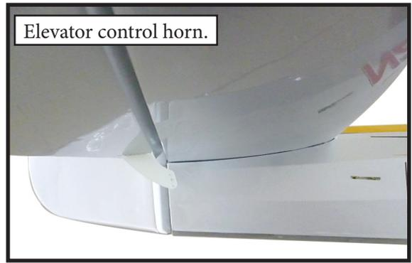
3) Thread one clevis and M2 lock nut on to each elevator control rod. Thread the horns on until they are flush with the ends of the control rods.
