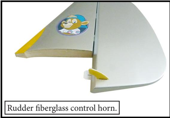
Rudder fiberglass control horn.
