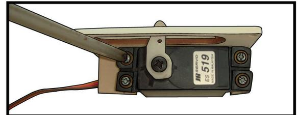
7) Apply 1-2 drops of thin C/A to each of the mounting tabs. Allow the C/A to cure without using accelerator.
