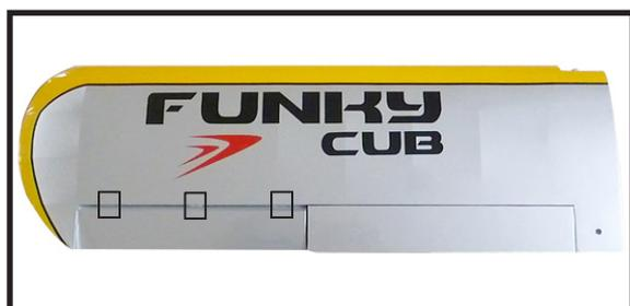
**Note :** Work the aileron up and down several times to “work in” the hinges and check for proper movement.
