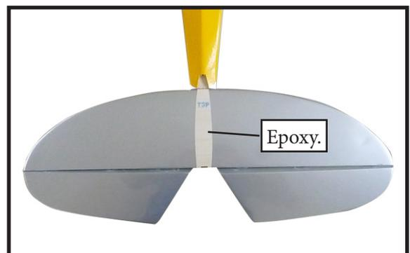
4) Slide the vertical stabilizer back in-place. Using a triangle, check to ensure that the vertical stabilizer is aligned 90° to the horizontal stabilizer.
