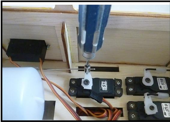
9) Move the throttle stick to the closed position and move the carburetor to closed. Use a 2.5mm hex wrench to tighten the screw that secures the throttle pushrod wire. Make sure to use threadlock on the screw so it does not vibrate loose.
