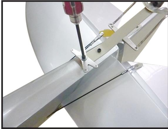
5) Install water rudder control cables.
