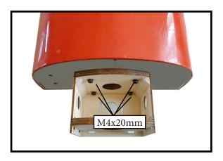
4) Attach the motor to the front of the electric motor box using four 4mm blind nut, four M3x12mm hex head bolts to secure the motor. Please see picture shown.
