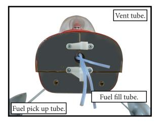
9) Connect the lines from the tank to the engine and muffler. The vent line will connect to the muffler and the line from the clunk to the carburetor.
