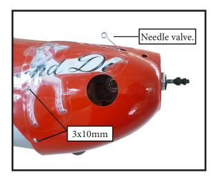
3) Slide the cowl in position on the fuselage. Use M3x10mm screws to secure the cowling to the fuselage.
