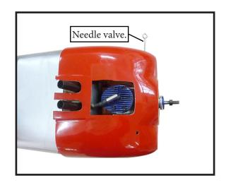
2) Slide the cowl in position on the fuselage. Use M3x10mm screws to secure the cowling to the fuselage.
