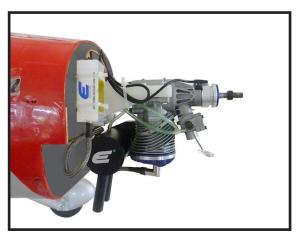
8) Reinstall the servo horn by sliding the connector over the pushrod wire. Center the throttle stick and trim and install the servo horn perpendicular to the servo center line.
