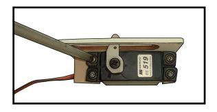
7) Apply 1-2 drops of thin C/A to each of the mounting tabs. Allow the C/A to cure without using accelerator.
