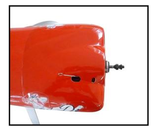
2) Carefully align the cowling on the airplane. The front of the cowl should be positioned so the crankshaft is in the middle of the cowl opening. Hold the cowl firmly in place using pieces of masking tape.
