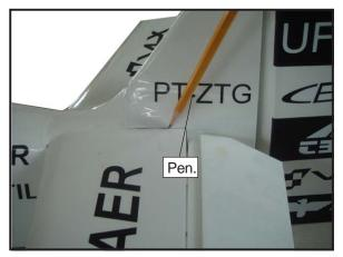
$\Box$  5) Remove the stabilizer. Using the lines you just drew as a guide, carefully remove the covering from between them using a modeling knife.
