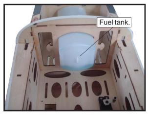
□ 8) Use plywood template to hold in place the fuel tank with C/A glue to secure the fuel tank inside the fuselage.
