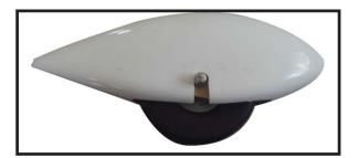
$\Box$  6) Slide the threaded end of the axle through the hole in the bottom of the landing gear leg. Use a washer and locknut to tighten the axle to the landing gear. Make sure to use threadlock on the nut so it won't vibrate loose in flight as shown.
