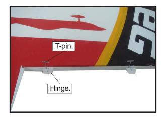
$\Box$  3) Slide the aileron on the wing panel until there is only a slight gap. The hinge is now centered on the wing panel and aileron. Remove the T-pins and snug the aileron against the wing panel. A gap of 1/64" or less should be maintained between the wing panel and aileron.
