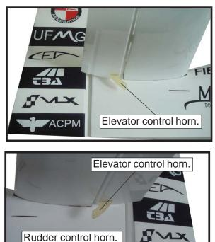
$\Box$  3) Thread one clevis and M3 lock nut on to each elevator control rod. Thread the horns on until they are flush with the ends of the control rods.
