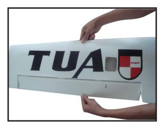
$\Box$  5) Turn the wing panel over and deflect the aileron in the opposite direction from the opposite side. Apply thin C/A glue to each hinge, making sure that the C/A penetrates into both the aileron and wing panel.
