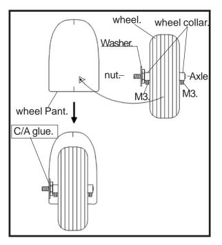
$\Box$  5) Place the wheel assembly in the wheel pants. The threaded portion of the axle will fit the notch of the wheel pant as shown.
