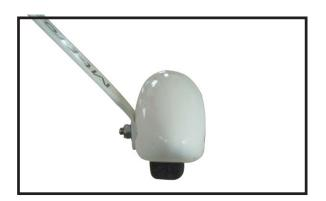
Repeat steps as above to attach remaining wheel pants to the landing gear.
