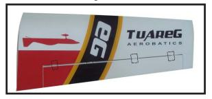
Note: Work the aileron up and down several times to "work in" the hinges and check for proper movement.
