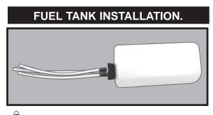
You should mark which tube is the vent and which is the fuel pickup when you attach fuel tubing to the tubes in the stopper. Once the tank is installed inside the fuselage, it may be difficult to determine which is which.
