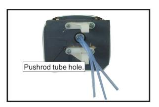
5) Slide the pushrod tube in the firewall and guide it through the fuel tank mount. Use medium C/A to glue the tube to the firewall and the fuel tank mount.
