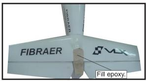
3) Slide the vertical stabilizer back in place. Using a triangle, check to ensure that the vertical stabilizer is aligned 90° to the horizontal stabilizer.
