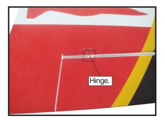
$\Box$  4) Deflect the aileron and completely saturate each hinge with thin C/A glue. The ailerons front surface should lightly contact the wing during this procedure. Ideally, when the hinges are glued in place, a 1/64" gap or less will be maintained throughout the lengh of the aileron to the wing panel hinge line.
