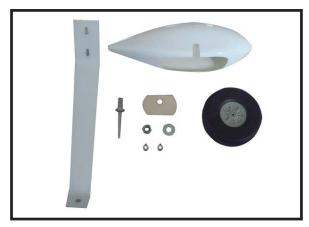
$\square$  2) Follow diagram below for wheel pant installation:Use a drill and 8mm drill bit to drill a hole in the wheel pants.
