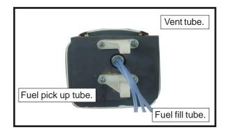
9) Connect the lines from the tank to the engine and muffler. The vent line will connect to the muffler and the line from the clunk to the carburetor.
