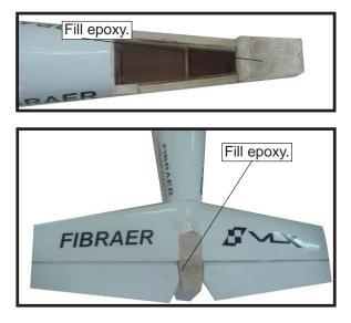
INSTALLING VERITICAL FIN.
