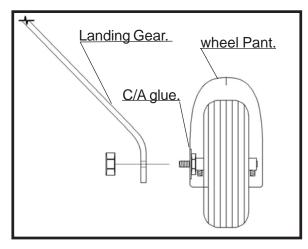
$\Box$  7) Tighten the setcrews using a hex wrench to secure the collars on the axle over the flat spot to retain the wheel as shown.
