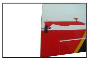
9) Set the aileron hatch in place and use a Phillips screw driver to install it with four wood screws.
